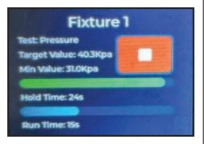
5. Press Enter or touch the Stop button on the touch screen to stop the test. The upper bar indicates the test pressure, and will be colored green if the pressure is within the acceptable range, or red if the pressure is outside the acceptable range. The blue-colored lower bar indicates the hold time.
