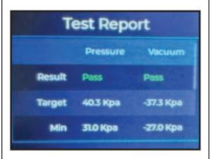
6. The device will generate a test report. Results in green are passing results, while results in red are failed results. Please make sure to scroll up and down to make sure you view the entire test report.
